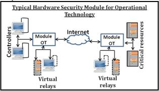
If such threats need to be addressed, then it may be wise storing the keys in a security module such as a smart card, an HSM or the TPM chip. Those modules ensure the protection of the cryptographic keys by only allowing operations on them and preventing their extraction. The purpose of the abstract key API is to provide an API that will allow the handle of keys in memory and files, as well as keys stored in such modules.
