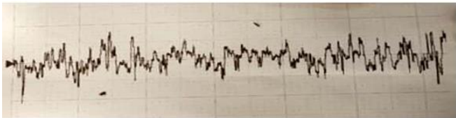
Fig 8. Final surface roughness
