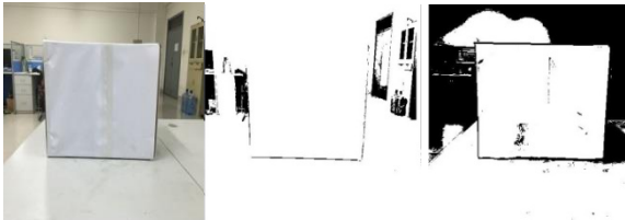
(a) original (b) fixed threshold (c) adaptive threshold Fig.8. Different threshold segmentation results
