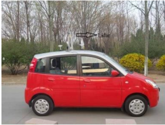
Fig.4 Experiment platform with lidar
