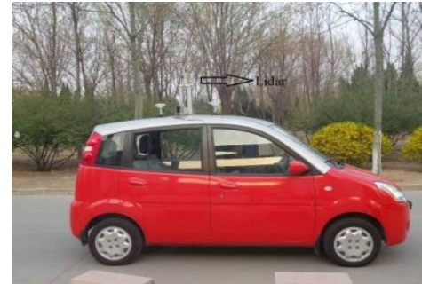
Fig.7 Experiment platform with lidar
