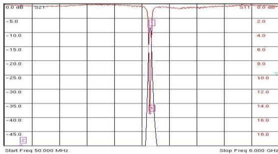
Fig.6 Measured reflection and transmission factor 50 MHz to 6 GHz.
