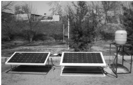
Fig.1. PV-T collector (right) and PV module (left) during the tests in Test Base of Physical-Technical Institute.
